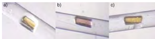
Figure 3. Photographs of a) original crystal 1 in the mother liquor, b) after evacuation of 1 at 150 °C and 10 −5 torr for 2 h ( 1' ), and c) after exposure of 1' to water vapor for 5 min ( 1'' ).
