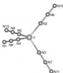
Figure 1. Predicted tetrahedral structure of free gaseous [\text{Ti}(\text{N}_3)_4] with linear \text{Ti}–\text{N}–\text{NN} bonds.
